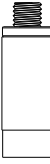
7B (ADP7992) Fit 15/16 Round Tube Exp. 0.900 - 0.980 Knurled Nut Round Rubber Round Plastic Bushing
